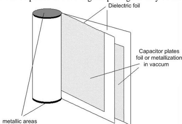
**Fig. 8** Capacitor with metallized foils (non-inductive)
