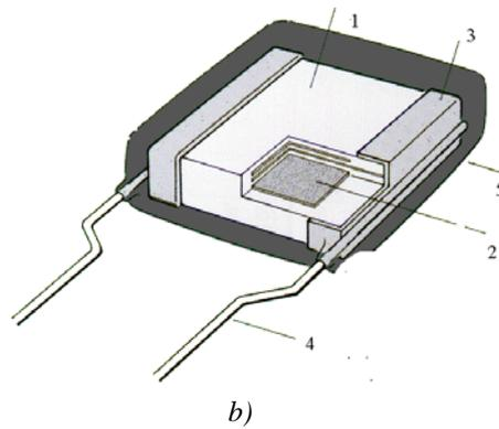
**Fig. 6** Multilayer ceramic capacitor: a) SMD technology, b) through hole.
