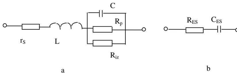
**Fig. 3** Equivalent circuit of the real capacitor.
