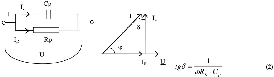
**Fig. 2** The loss angle.
