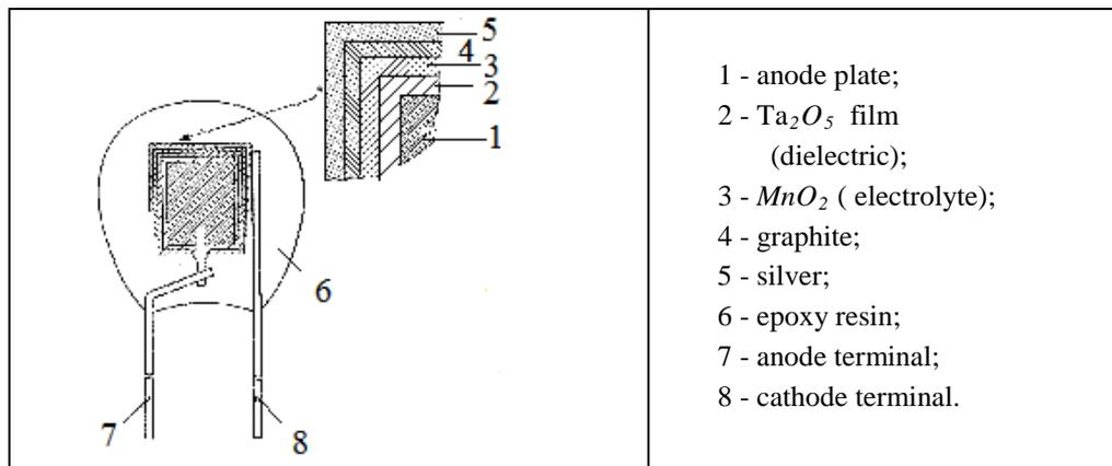
**Fig. 10** Constructive structure of electrolytic tantalum capacitors, with solid electrolyte, drop type
