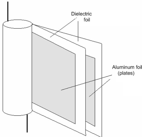
**Fig. 7** Capacitor with aluminum foil
