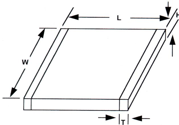
**Fig. 11** Dimensions of a rectangular SMD chip type capacitor
