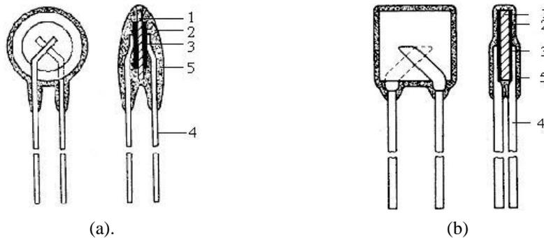
Fig. 5 Single-layer ceramic capacitor. (a) disk, (b) a flat capacitor.
