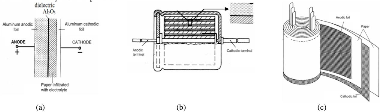
**Fig. 9** Aluminum electrolytic capacitors
