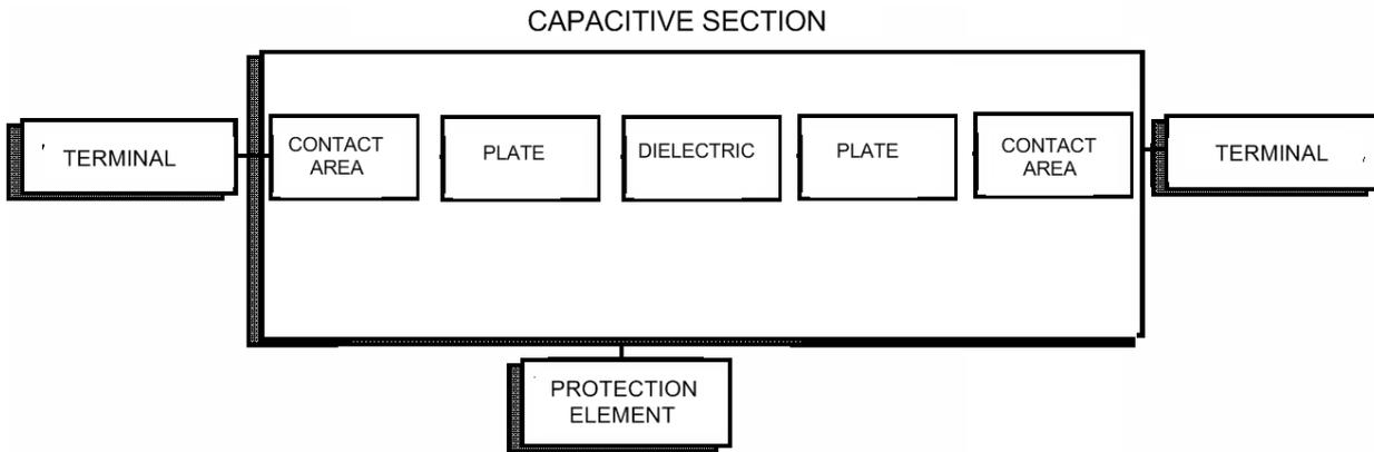
Fig. 4 The constructive structure of capacitors.
